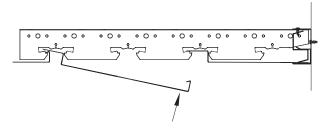
**3.21.4** Cut the fingers off of a splice plate and secure it into the end of the installed panel with a piece of two-faced tape.
