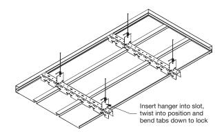
**3.8** Fasten the carrier to the molding at the proper location, align the notch as indicated in Section 3.6 and fasten with a framing screw or pop rivet. Notch the carrier to fit into the wall molding as needed.
