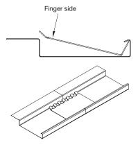
Panels 12" wide have a factory return on the ends and have two options to splice the panels when they do not reach across the space in one piece. Install panels so the factory joint is tight and use vise grip pliers to temporarily hold together.
