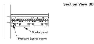
The end of the panel will fit into the molding channel on the adjacent wall. A pressure spring is required on the end of all 8" wide panels that rest on the wall molding.
