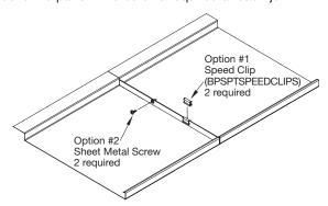
Note: Ends of installed panels will always be visible with this system.
