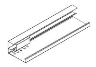
**3.16** Cut the panels to length to fit into the perimeter molding at the sides, parallel to the carrier. Cut end will fit into the lower channel. Use pressure springs on ends as needed.
