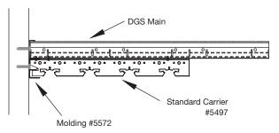
**7.5.6 Install panels:** Measure, cut, and install the first border panel as described in standard MetalWorks Linear instructions. Install pressure spring (item 5576) every 12" along the border panel.
