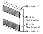
For full size Woodworks Tegular panels using 9/16" grid, cut a miter on each end of each side of the trim so the inside dimension is 1-3/16" larger than the nominal dimension.
