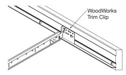
When a full sized XL cross tee meets the molding at the perimeter, line up two holes in the Trim Clip with the two "stake" holes in the end of the cross tee.
