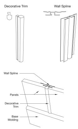
If the trim does not protrude from the face of the panel, cut the trim so it rests on the ground strip at the bottom and extends to the top of the panel.
