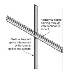
The installation of the ground strip, baseboard and finish molding is done the same as with vertically mounted panels. Remember to cut horizontal accent trims that protrude from the face of the panels 3/8" short of the end of horizontal panels. This will accommodate the fit of the finish molding installed vertically at the end of the installation.
