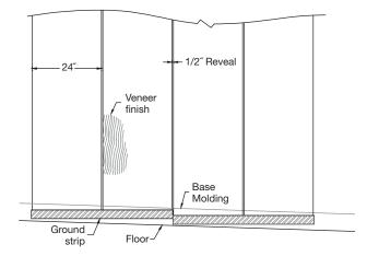
**2.2.1** Install 3/4" thick lumber (by others), aligning the top of the lumber with the level line. The width
