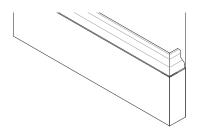
Fasten the quarter round molding to the base molding at the floor to close off any openings due to the unevenness of the floor.
