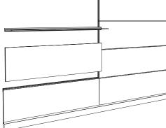
Vertical splines can be secured to the wall using appropriate fasteners. The vertical splines capture the vertical edges of the panels. The horizontal and vertical splines must meet at a 90-degree angle.
