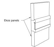
Predrill and countersink holes for flat head screws in the insert channel of the Mounting Rail.
