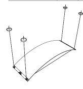
FOR EACH HANGING KIT THAT IS SPECIFIED. INCLUDE ONE ESCUTCHEON KIT TO PROVIDE A COVER FOR THE HOLE CREATED IN THE EXISTING CEILING.
