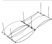
Four canopies linked and suspended with one cable at one end of each canopy, and one dual canopy cable between end-linked canopies, you need:
