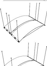
Two canopies (2' x 5', 2' x 6' or 4' x 10') linked and suspended with two cables on each side, you need:
