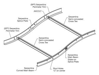
Serpentina Perimeter Trim Clips (AXCCLT Clips) are used for the attachment of grid (Main Beams & Concealed Tees) to the Serpentina Perimeter Trim. Hold the insertion tab with pliers and twist to lock into place.
