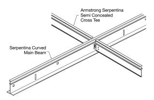
**8.3.** Attach the StrongBacks to the cross tees by inserting screws through the holes provided near each end of each tee.
