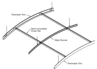
**2.2.** Installations that are 6' wide or greater are to be supported from the main beams as follows (see final assembly drawings on page 5):
