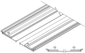
Serpentina WAVES Connector Sleeve (SPTCS4-12) is a PVC extrusion that slips over the flange of the main beams. The panel hangers, mounted on the back side of the panels, slide into the grooves on the sleeve. The main beams are completely concealed from view when the panels have been installed.
