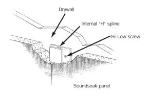
2.7 When installing Soundsoak around door or window frames, there are two options for handling edge treatment. Use either a "J" Molding or a fabric-wrapped edge as previously described in Step 3. Around receptacles, follow standard electrical codes. Anytime the back of a panel is cut or scored, apply a heavy nonporous tape or foil to reseal the back to prevent air flow through the panel which can cause soiling of the fabric surface.
