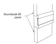
Mineral fiber Soundsoak 60 wall panels fit above and/or below the chair rail and rest in the channel on the top and/or bottom side of the Mounting Rail.
