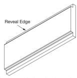
NOTE: The Rail Insert with the aluminum face can only be applied visually as a flat side and can be secured to the rail with double-faced tape (by others). The aluminum Rail Insert has a protective film on the face that should be removed before securing to the rail.
