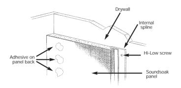
**2.6** Cut the next panel to length and insert the lead edge into the previously attached "H" spline, insert another spline into the trailing edge, and attach to the wall as before. Proceed progressively along the wall as described.
