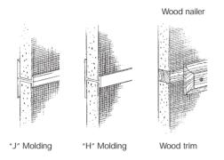
**2.11** Apply "J" Molding to the top of the panels. Apply any other finish trim desired such as cove molding or wood molding.
