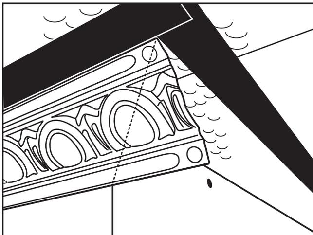
Cut the molding with snips. Do the same for the other side of the corner using another piece of cornice. Check the fit of the two pieces. Trim and fit the two pieces until the joint makes a satisfactory appearance. Use these pieces as templates for marking and cutting the actual pieces that will be installed. If the moldings will be painted, fill the joint line with caulk. If the moldings will be left unpainted, file the joint until it fits. It takes time and patience to make a good fit.
