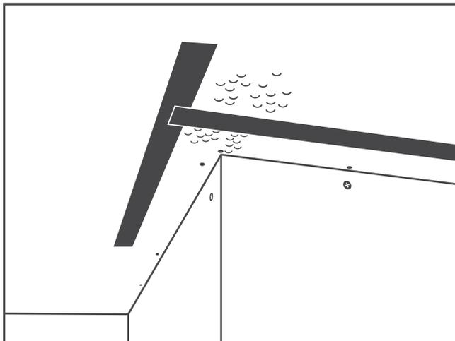
Hold a piece of cornice against one wall aligning it with the tape on the ceiling. Let it extend out past the corner and past the intersecting masking tape. Mark the molding at the bottom where it intersects the corner, and at the top where it meets the tape intersection. Draw a line to connect these two marks.
