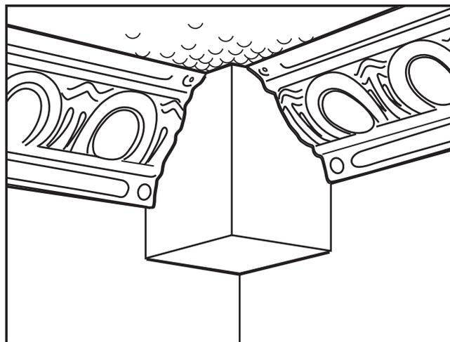
You can also cope inside corners. Butt one piece into the corner. Then trim the second piece on the adjacent wall to fit. First place a strip of masking tape across the end of a scrap piece of molding. Hold the scrap molding in the corner and use a compass or scribing tool to transfer the profile of the nailed-in-place piece to the scrap piece.
