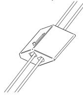
Securely tighten the cables by pulling on the free end. Make sure that the spine remains level in both directions and that all slack is removed as the cables are secured.
