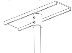
**WARNING**: This system and the supplied cables are designed around a maximum conduit length of 10<sup>'</sup>. Consult an engineer for guidance when greater drops lengths are desired.
