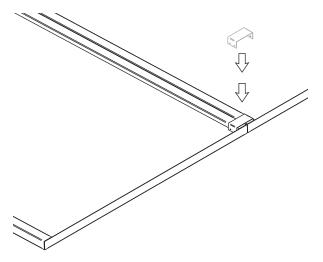
Each panel-to-panel joint MUST have an alignment clip installed.
