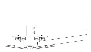
**WARNING**: Check to ensure that the panel notch has engaged the vertical rib located at the back of the channel.
