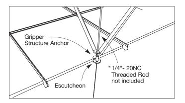
Use the optional escutcheon kit accessory to conceal the structure gripper anchor when installed above the ceiling level.
