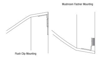
NOTE: Location of the clips along the panel edges is not critical. However, if the following measurements are used, locating the mating wall clips will be much easier. Position the outer edge of each clip on the top edge of the panel 1" in from the corner of the unit. When wall clips are to be used to secure the bottom edge of the units, position them with the lower edge of the clip 2" up from the bottom corner of the unit. Location of clips with mushroom fasteners is not critical.
